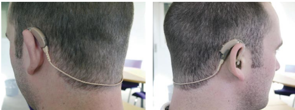
Figure 2. A CROS adaptor on the left ear and a hearing aid with an audio shoe on the right ear; a CROS adaptor cable connects the two units.
